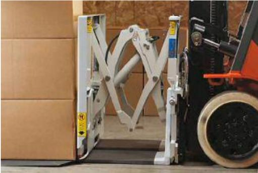
1. Position the load over the unloading point (truck deck)
