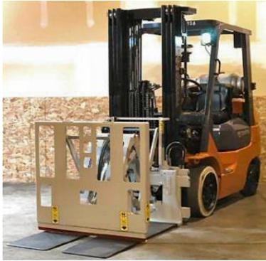
Push/Pull Attachment must be fitted to the Forklift
